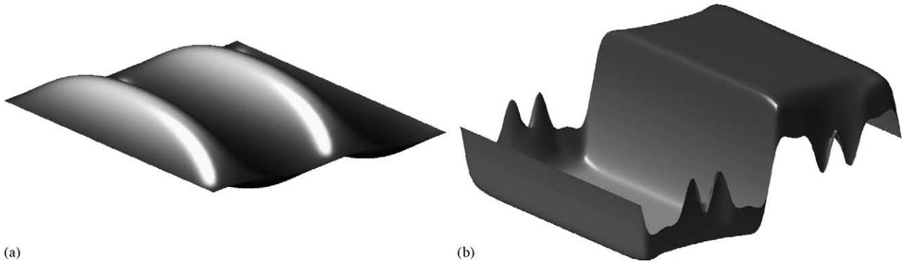
Fig. 2. Polarization profile (a) for soft domains ( $2a_f = 700$  nm,  $T = 0$ ) and (b) for hard domains ( $2a_f = 100$  nm,  $T = 0.7T_c$ ). The scales in different directions are not proportional.
