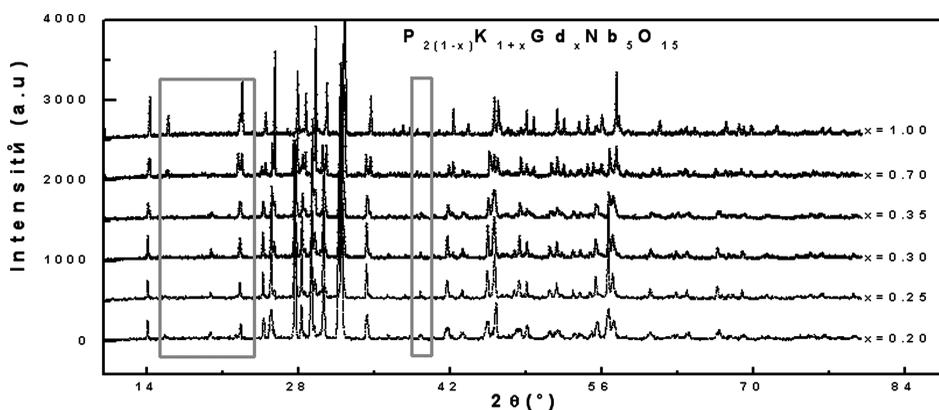
Figure 1. X-ray diagrams of the PKGN compounds.
