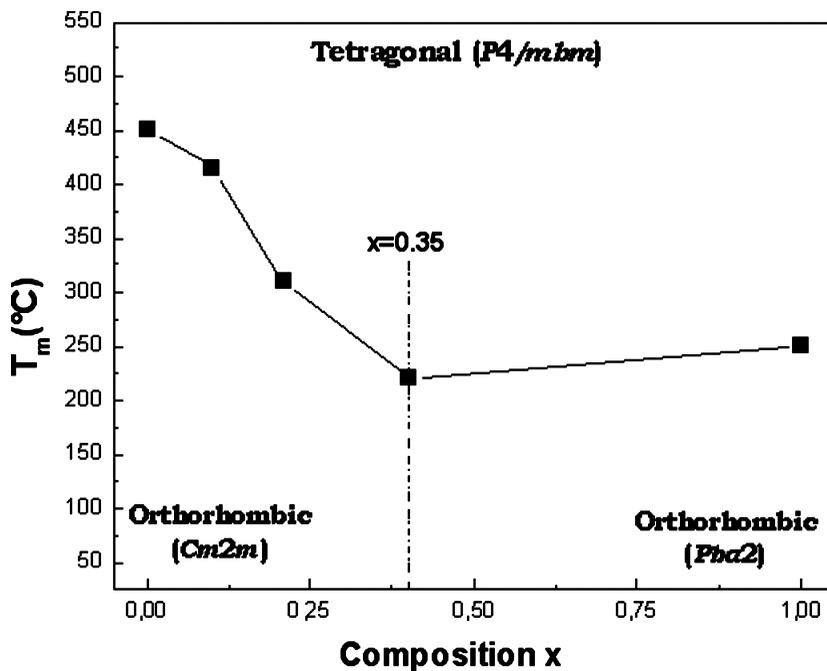
Figure 4. Proposed phase diagram of PGKN compounds.
