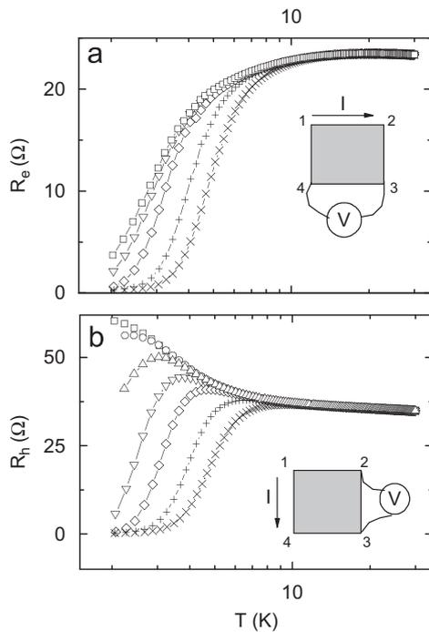
Fig. 1. Temperature dependencies of resistances measured in “easy”  $R_e = V_{34}/I_{12}$ , (a), and “hard”  $R_h = V_{23}/I_{14}$ , (b), directions for  $I_{12} = I_{14} = 10 \mu\text{A}$  and frequencies: (a)  $f = 10, 100, 200, 500, 1000 \text{ Hz}$ ; (b)  $f = 10, 25, 50, 100, 200, 500, 1000 \text{ Hz}$ , from top to bottom.
