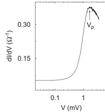
Fig. 2. Differential conductance  $G \equiv dI/dV$  vs.  $V$  dependence measured at  $T = 5 \text{ K}$  and  $f = 60 \text{ Hz}$  in “hard” direction;  $V_p$  marks the maximum in  $G(V)$ .
